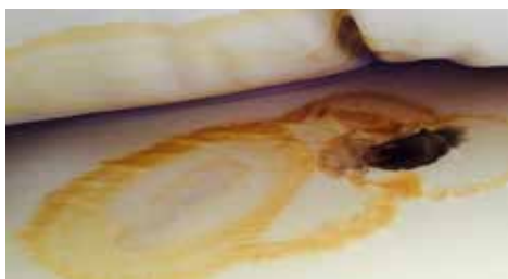
Contamination of foam as a result of strike-through in mattress cover
